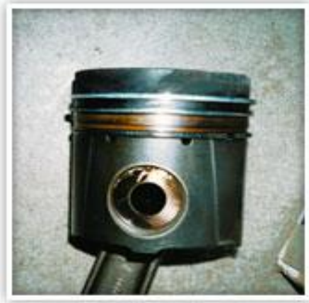
Cummins piston as removed from engine after 15,000 hrs use on FTC Decarbonizer treated fuel.
