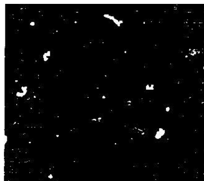
Particulate emissions from diesel exhaust with FTC Decarbonizer ( 849 \times 10^6 Particles / m^3 )
